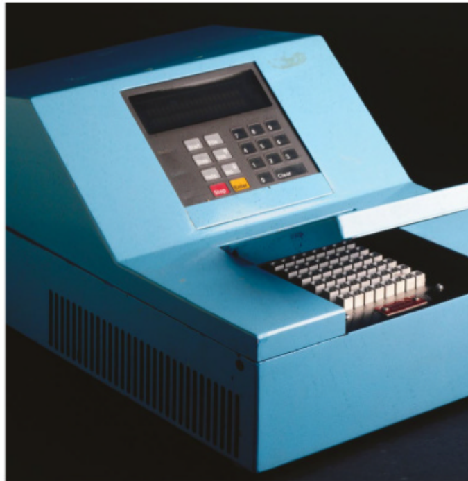
○ This device is a prototype of one of the first DNA-photocopying PCR machines of the 1980s
