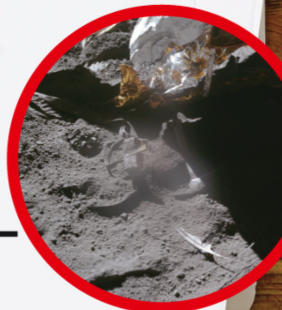
○ Under the near vacuum conditions on the Moon the hammer and feather fell at the same rate
